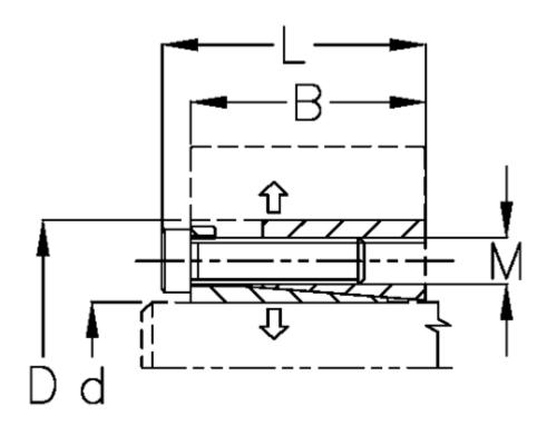
$\begin{array}{lll} \text{B mm} & = 64.0 \\ \text{d H8 mm} & = 200 \\ \text{D mm} & = 260 \\ \text{Fit tolerance} & = \text{Aksel h8, Nav H8} \\ \text{F kN torque} & = 600 \\ \text{L mm} & = 78 \\ \text{M mm} & = \text{M14} \\ \text{P N/mm2 surface pressure on shaft/hub} = 140 \\ \end{array}$
